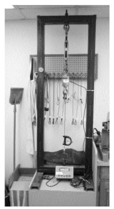
Device used for tension meter calibrations
