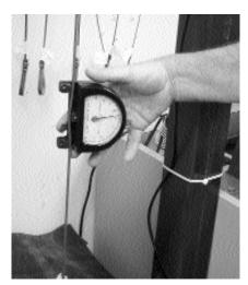
Calibrating a cable tensiometer
