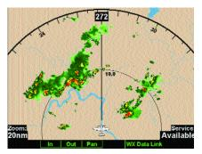
NEXRAD graphic as seen via the Capstone Universal Access Transceiver (UAT) data link system.
