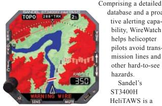
WireWatch has been added to Sandel's ST3400H HeliTAWS terrain avoidance system.
