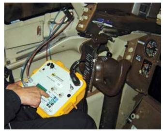
DMA-Aero's MPS43 Ultra Compact Air Data Test Set weighs 9 pounds.
