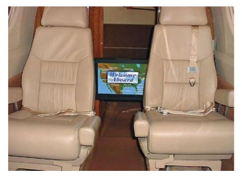
A King Air 200 with Flight Display Systems' 17-inch HD LCD slide mount.
