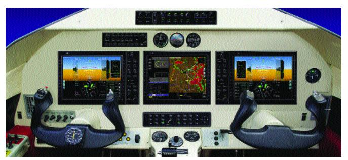
Honeywell's APEX integrated avionics suite
