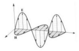
Figure 1 The E and H vectors in a plane electromagnetic wave, traveling along the positive x axis. The field vectors are mutually perpendicular and are in phase.
