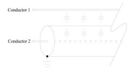
Figure 3 Adding a shield significantly reduces capacitive coupling.
