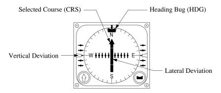
Figure 1 Typical Horizontal Situation Indicator (HSI).
