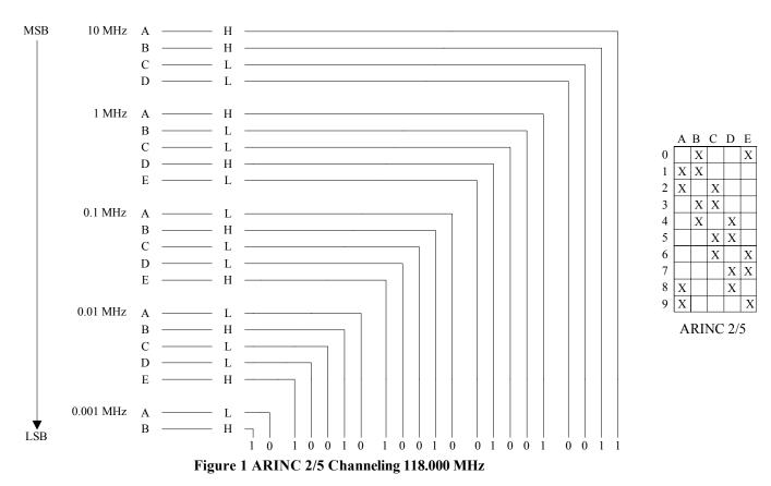
Below, in Figure 1, is the wiring diagram utilizing ARINC 2/5 channeling for 118.000 MHz:
