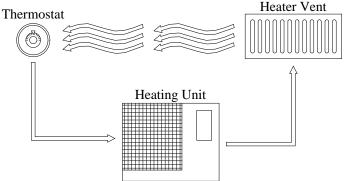
Figure 1 Furnace shown as example of feedback loop.
